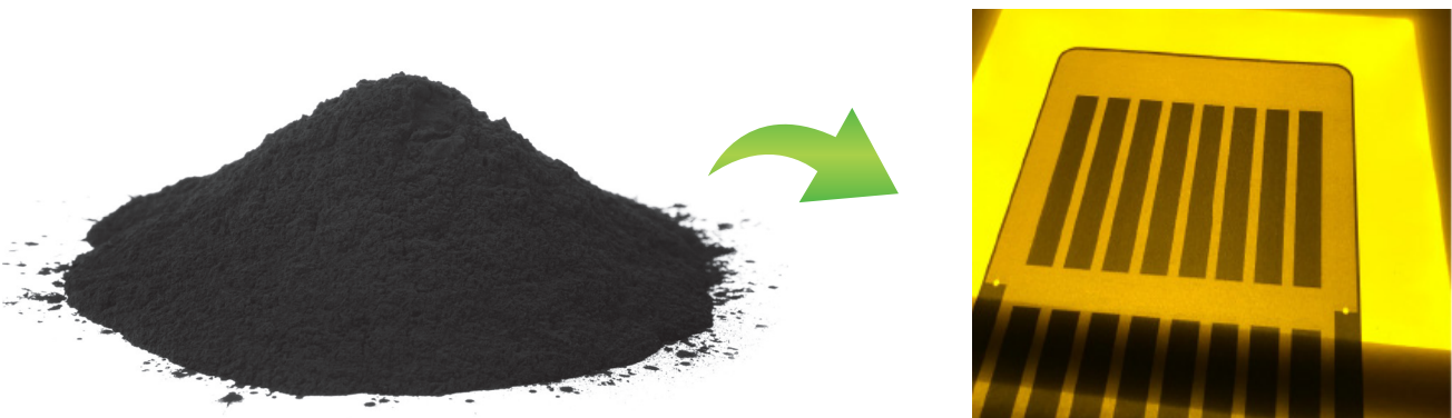
Left, ABS toner particles. Right 1 layer of ABS part and support particles
